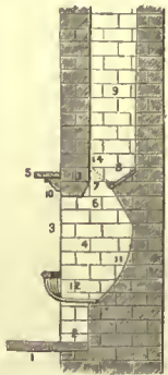
Section of Fireplace. 1, slab; 2, hearth; 3, jamb; 4, fireplace; 5, mantelpiece; 6, throat; 7, gathering; 8, funnel; 9, flue; 10, mantel; 11, back; 12, grate; 13, breast; 14, damper.
